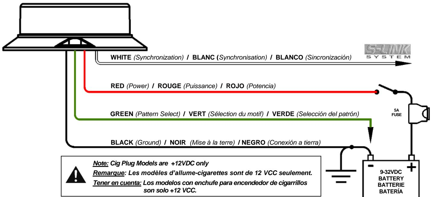
**CAUTION !!** All of our DC powered warning lights are polarity sensitive. These lights are polarity protected *only if the appropriate fuse is used*. All wires connected to the positive terminal of the battery should be fused *at the battery* for their rated load. **Testing the light before this fuse is properly installed will void the warranty on the light.**
